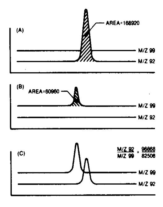
FIGURE 6 Extracted Ion Current Profiles for (A) Toluene, (B) Toluene-d<sub>a</sub>, and a Mixture of Toluene and Toluene-d<sub>a</sub>.
