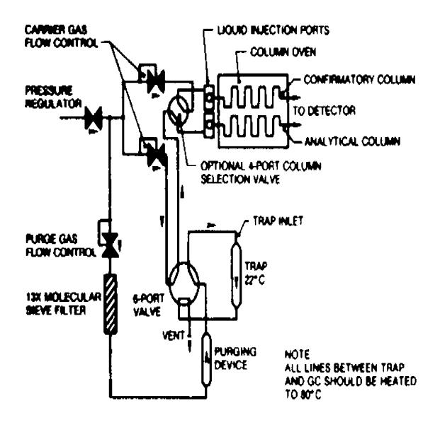
FIGURE 3 Schematic of Purge and Trap Device—Purge Mode.
