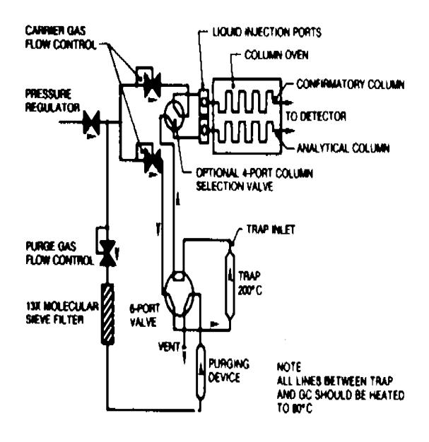
FIGURE 4 Schematic of Purge and Trap Device—Desorb Mode.
